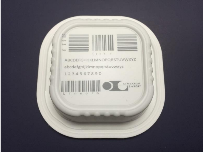
Figure 7. Image of the printed content directly applied to the plastic container, including a 1D readable bar code. All font sizes were readable as well.
