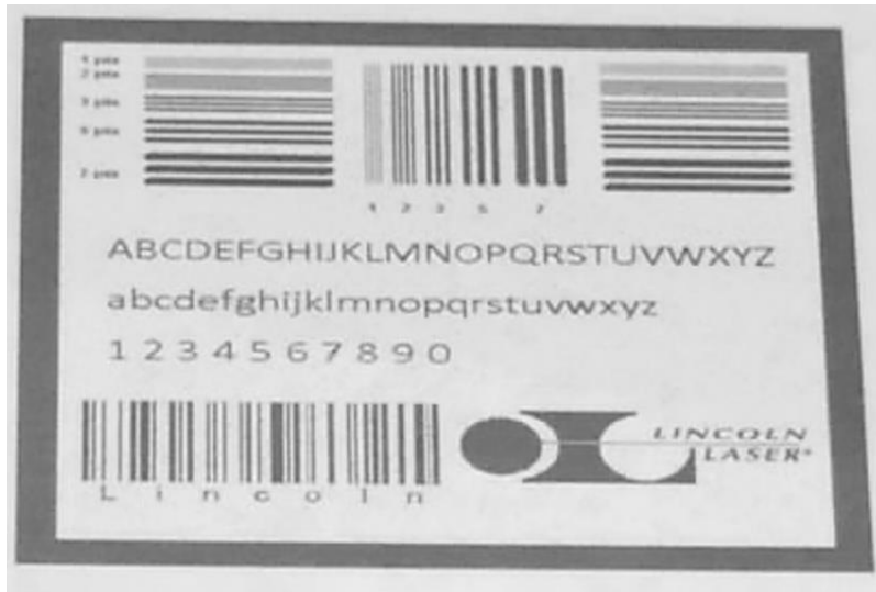
Figure 4. Image of the typical test content as loaded into the Lincoln Laser POLYtek™ high speed polygon scan head test program. The content was converted into a bitmap file and then loaded into the program via the user control panel.
