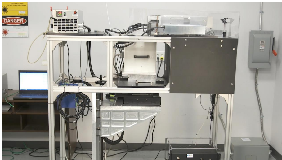
Figure 2. Side view of the typical test configuration in the Lincoln Laser lab. The Lincoln Laser POLYtek™ high speed polygon scan head is shown placed in the middle section of the test frame. An f-theta lens is facing downward toward the test bed table which is located directly below it. The target is lying on the test bed below.
